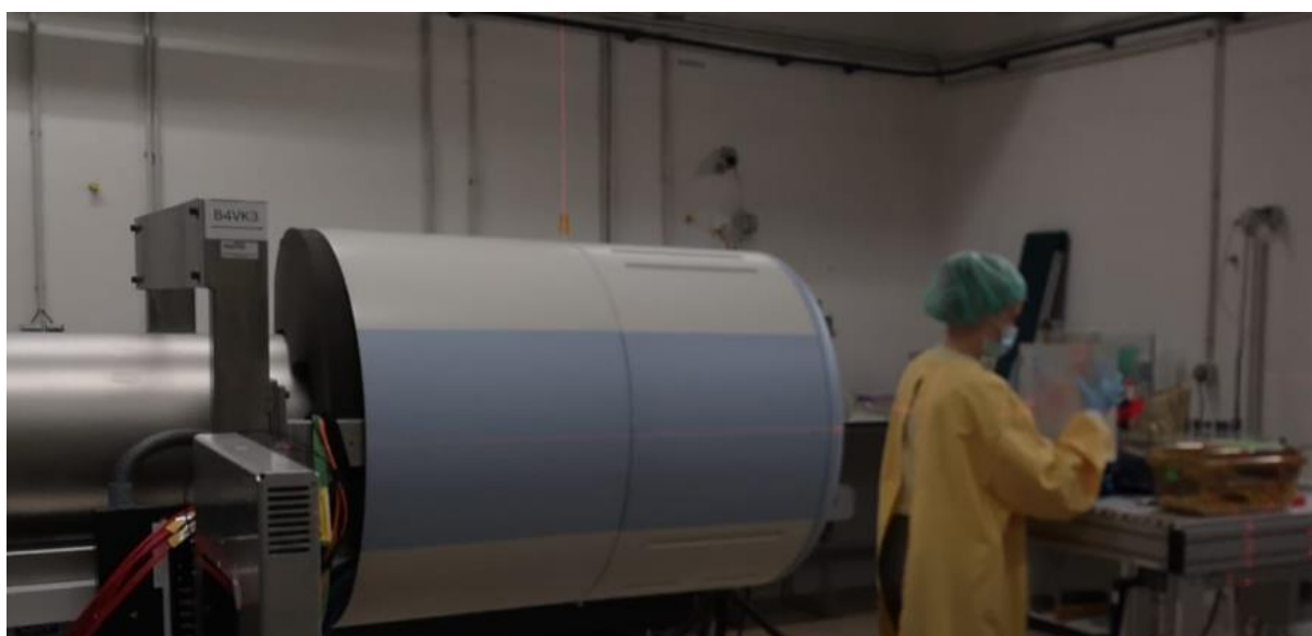
Figure 2: Vertical beam set-up for proton and carbon irradiation at the Heidelberg Ion-Beam Therapy Center (HIT).
